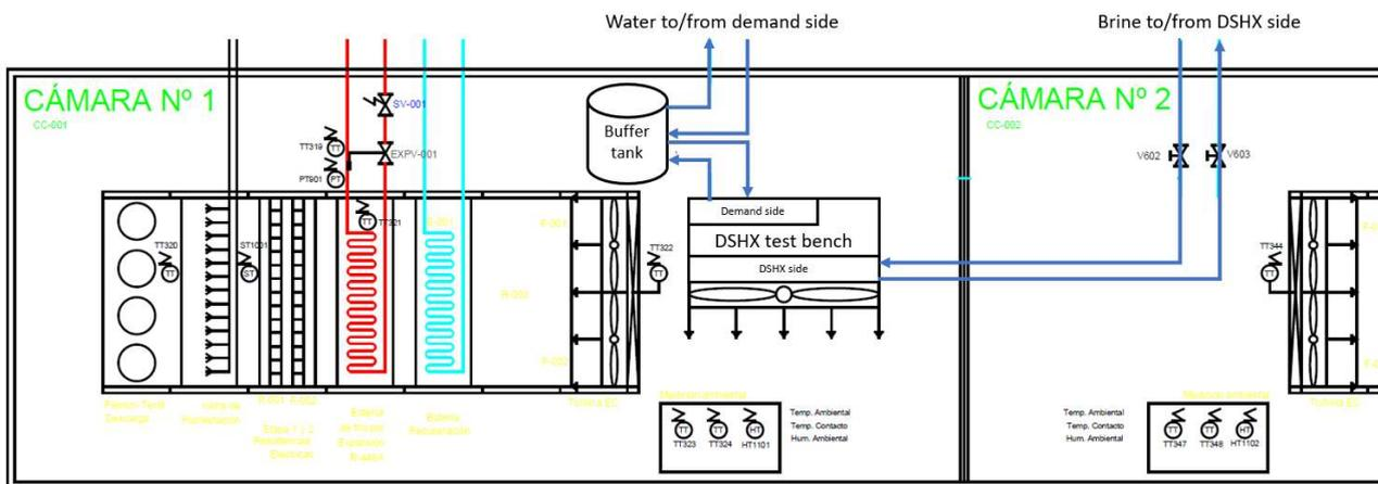
Figure 8. Scheme of the DSHX test bench installed in the climatic chamber.
