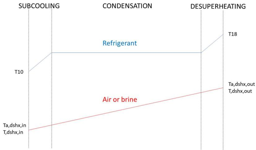
Figure 12. DSHX working as a condenser (Cooling mode). Refrigerant can exchange heat with air, brine or both at the same time.
