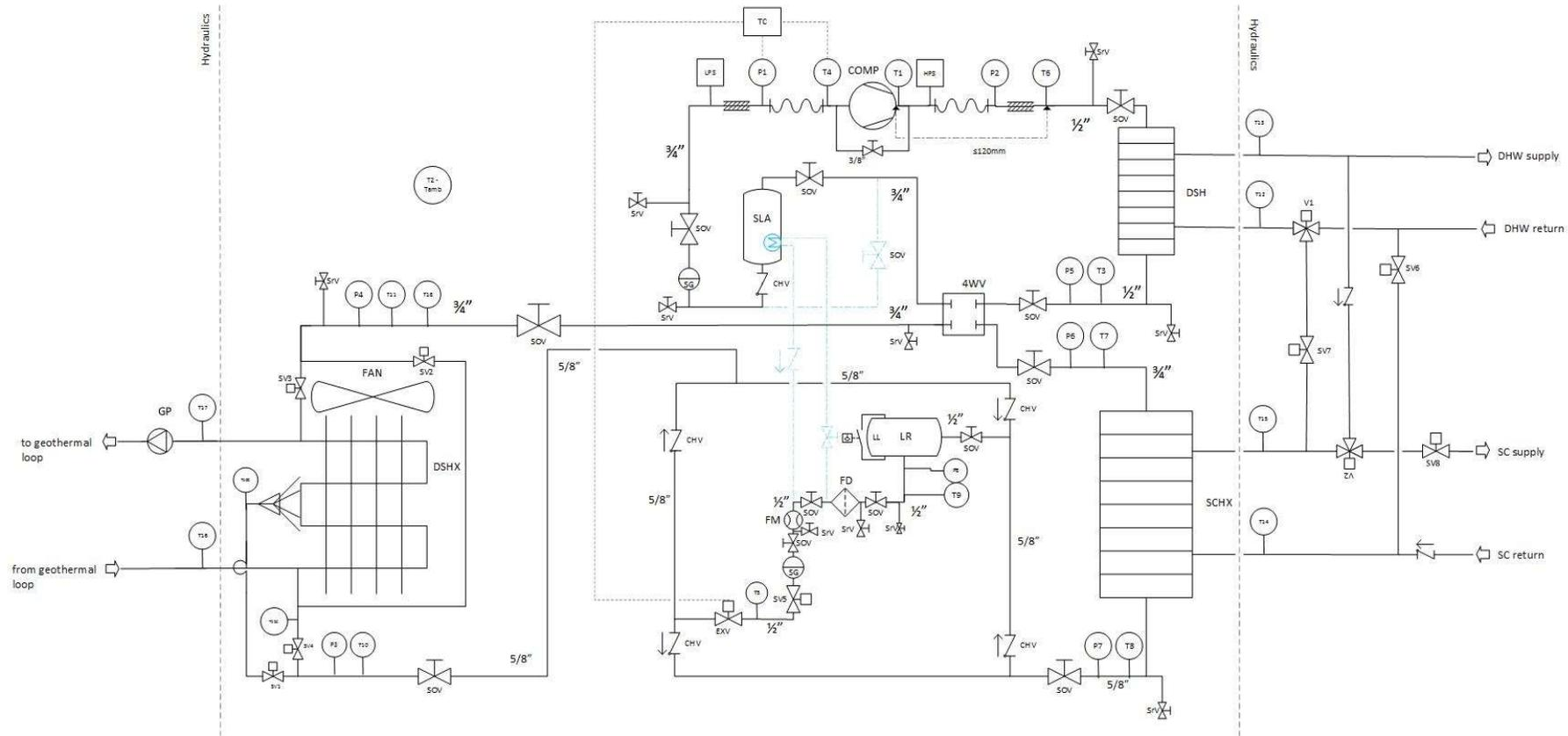
Figure 1. DSHX test bench P&ID.
