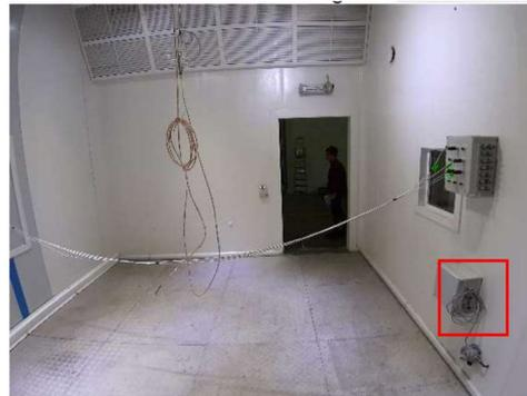
Figure 4. Leak detection sensor and location inside Climatic chamber.
