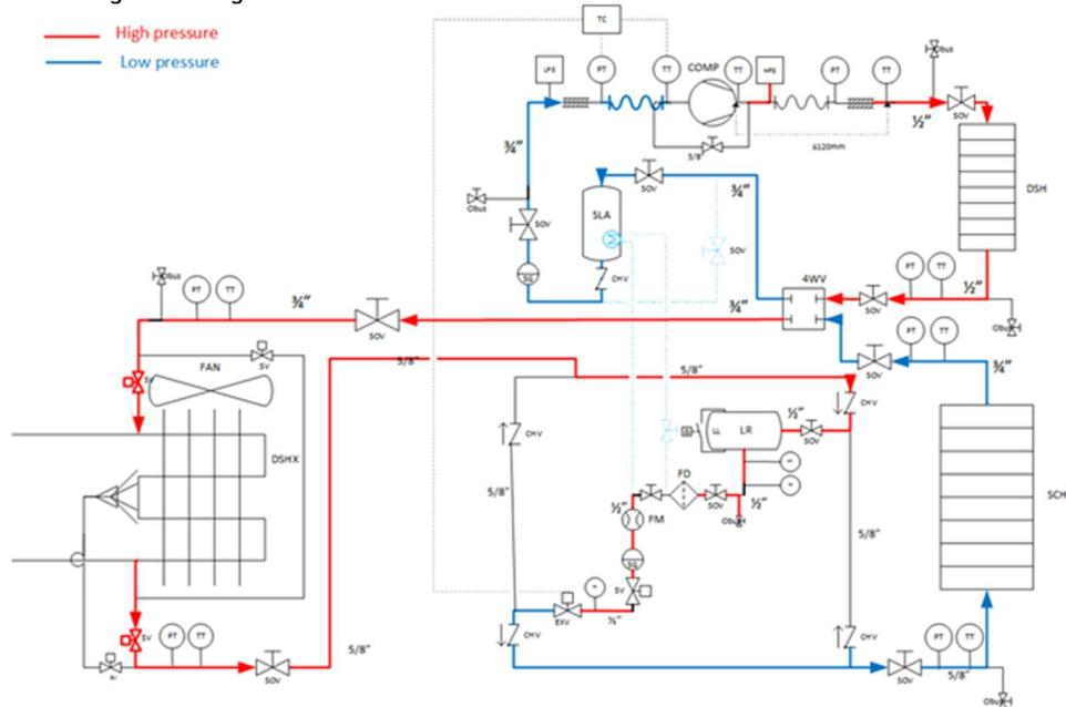
The circuit between the DSHX and the SCHX includes several check valves, in order to assure the correct circulation of the refrigerant in both working modes, going first to the liquid receiver and then to the expansion valve. A filter drier, Coriolis flow meter and sight glass are included after the liquid receiver and before the expansion valve.
