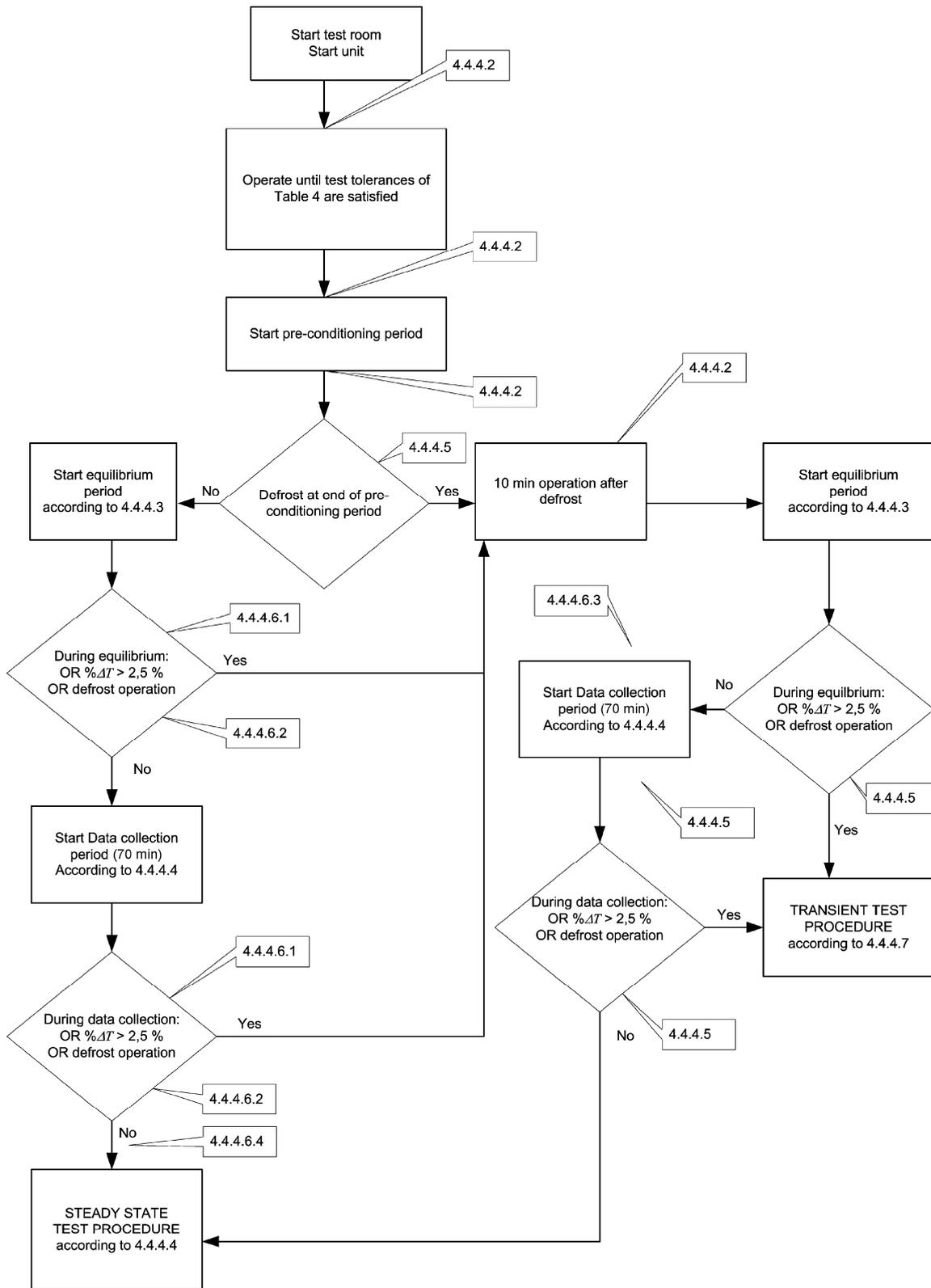
Figure 10. Flow chart of test procedure according to EN 14511.
