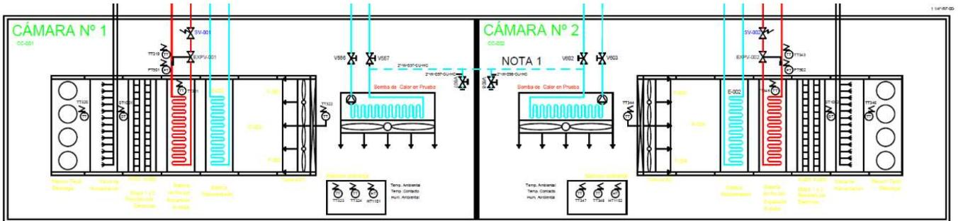
Figure 6. Hydraulic circuit of the climatic chamber.
