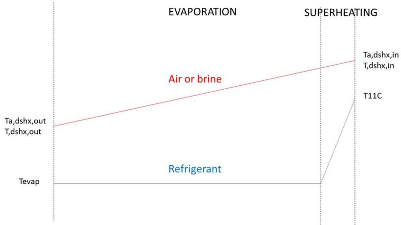
Figure 11. DSHX working as an evaporator (Heating mode). Refrigerant can exchange heat with air, brine or both at the same time.
